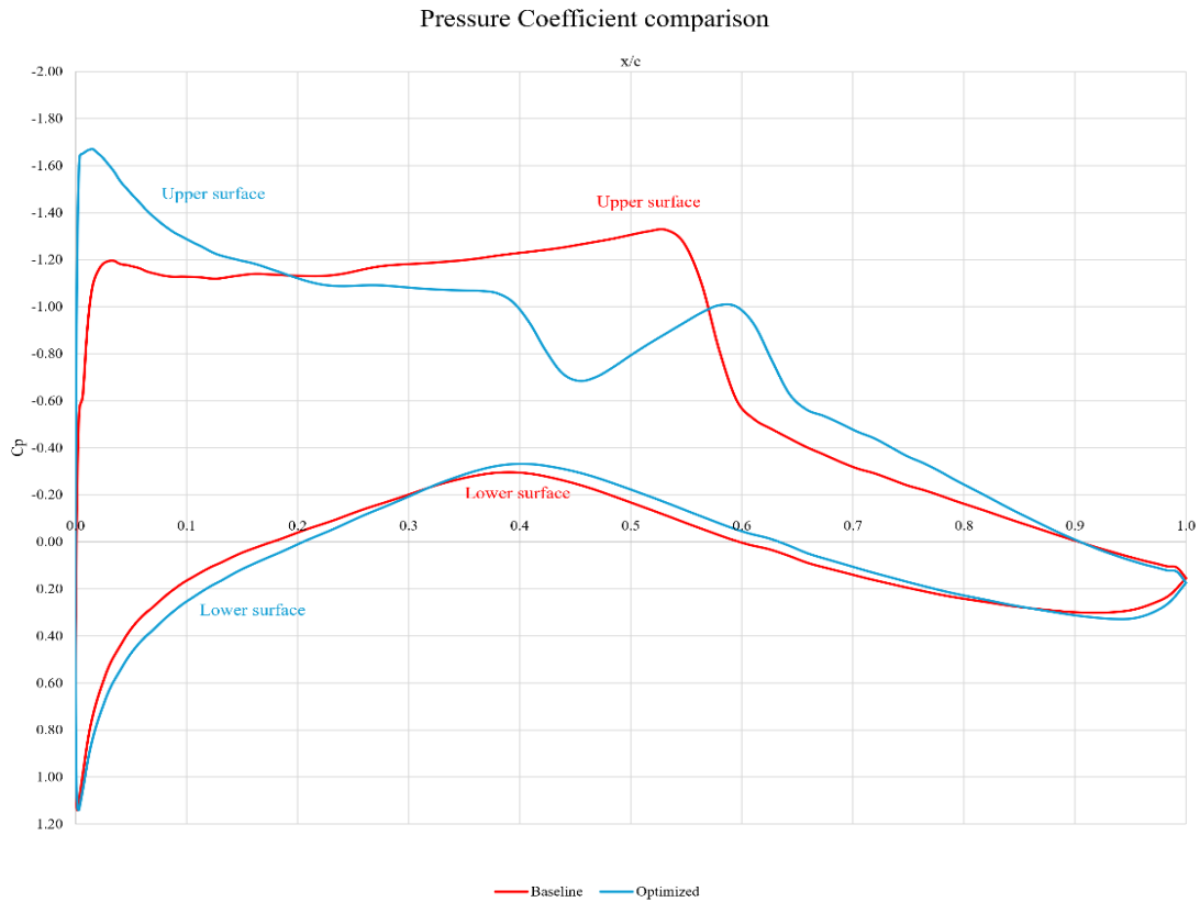
Figure 85. Pressure coefficient comparison between baseline and modified geometry for Study Case 3 (wrong C_m definition).
