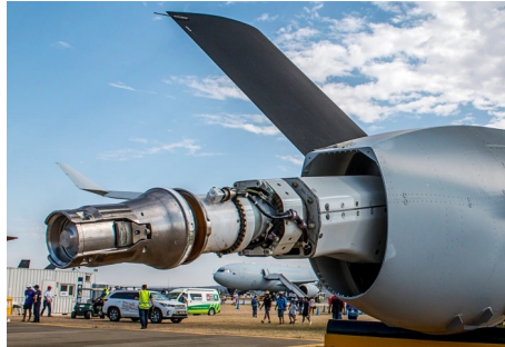
Figure 4.7: Fuel transfer nozzle in a real operating tanker aircraft (Yonhap News Agency, 2019)
