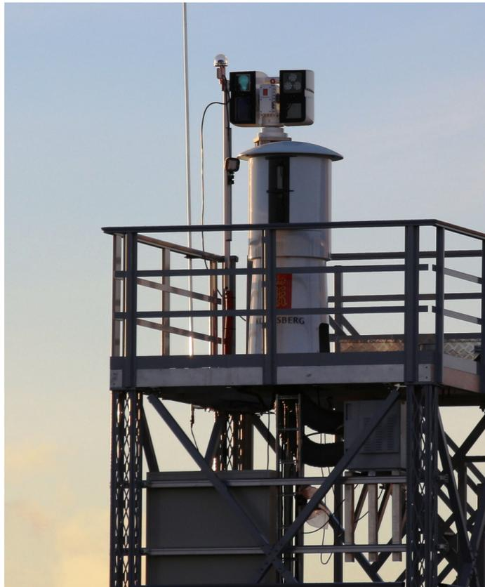
Fig. 3.1. Concepto de las cámaras de control remoto. Disponible en:<https://www.kongsberg.com/globalassets/kongsberg-defence--aerospace/2.1.-products/defence-and-security/aviation-and-security/remote-and-digital-towers/kongsberg-remote-towers.pdf>. [Accedido el 10 De Febrero]
