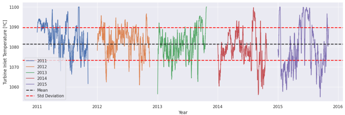
Figure 4.39: Turbine inlet temperature seasonal plot with Savitzky-Golay filtering (showing mean and standard deviation)
