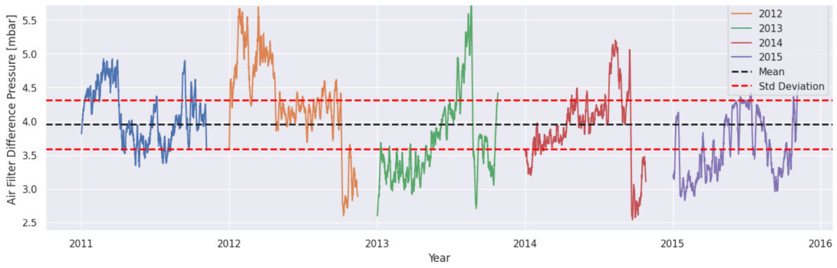
Figure 4.37: Air filter difference pressure seasonal plot with Savitzky-Golay filtering (showing mean and standard deviation)
