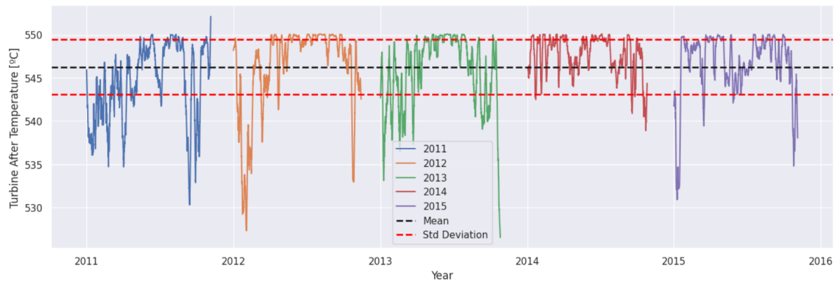
Figure 4.40: Turbine after temperature seasonal plot with Savitzky-Golay filtering (showing mean and standard deviation)
