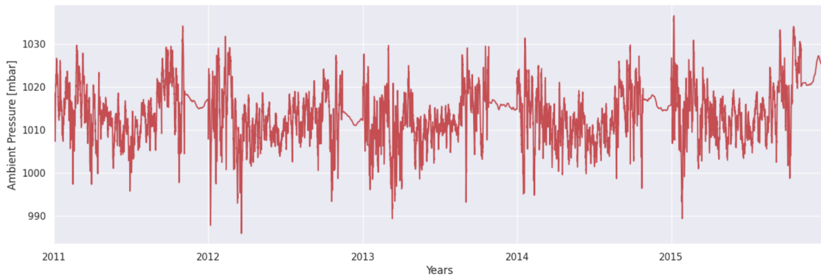
Figure 4: Ambient pressure graph obtained with KNN mean (n=2920) method for filling missing values
