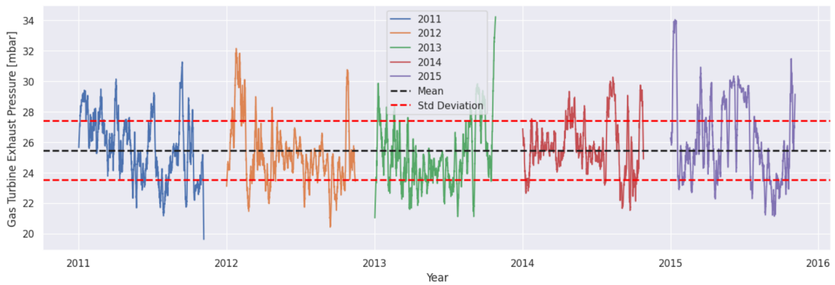
Figure 4.38: Gas turbine exhaust pressure seasonal plot with Savitzky-Golay filtering (showing mean and standard deviation)
