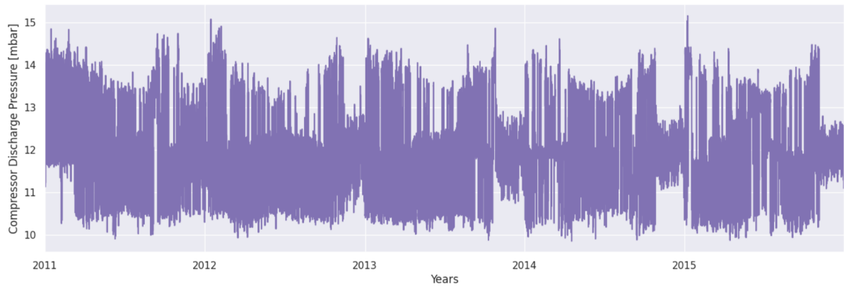
Figure 31: Compressor discharge pressure graph obtained with seasonal mean (n=2920) method for filling missing values
