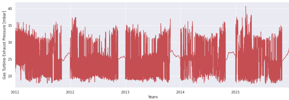
Figure 16: Gas turbine exhaust pressure graph obtained with KNN mean (n=2920) method for filling missing values
