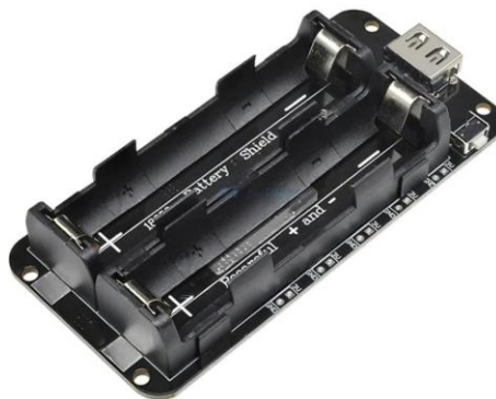
Figura XI Battery Shield V8. Fuente "eledelitio"
