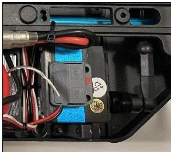
**Figura 28:** Servo motor Carson
