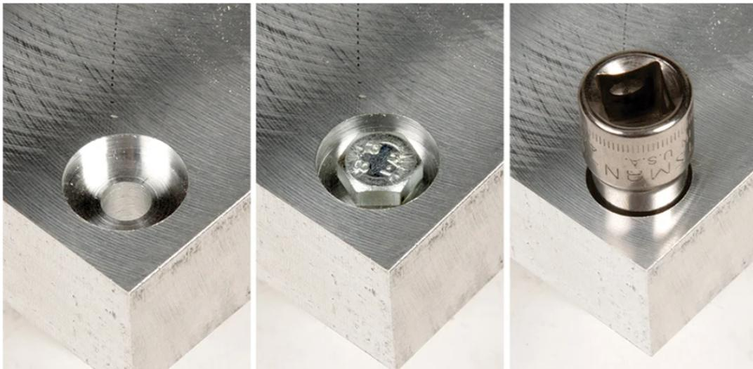
Figure 1.14: Fastener and socket installed with hole clearance
