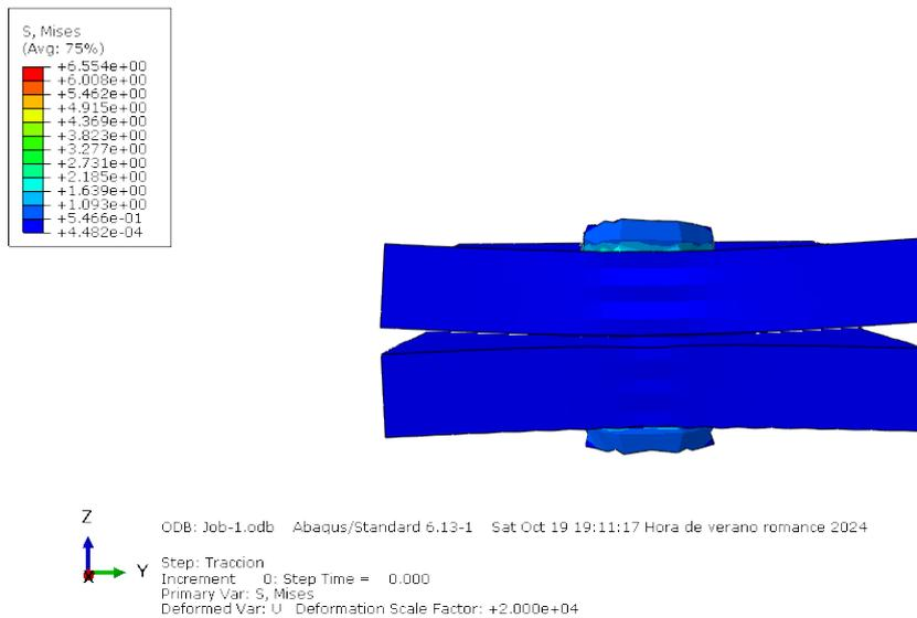
Figure 3.19: Plates bending during pretension (y-z plane)
