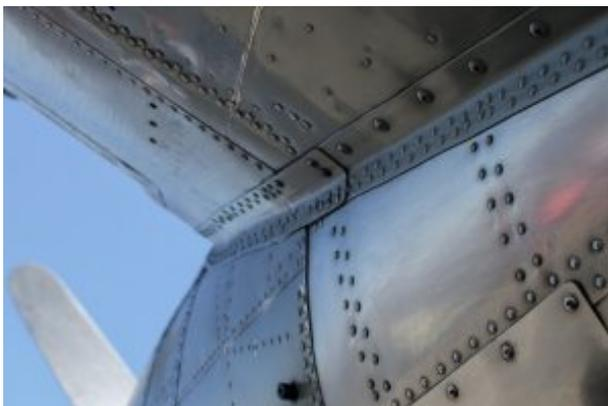
(a) Riveted fuselage panels
